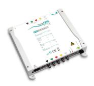
Optical transmitter for distribution of up to 4 satellites on a single fiber with CWDM (Coarse Wavelength Division Multiplexing) technology. Innovative solution to transmit the entire TV band, including radio signals, and an entire orbital position on a single fiber. 7dBm with FP SAT+TV+FM laser, wavelength 1310nm. (dimensions 230x230x50mm)
